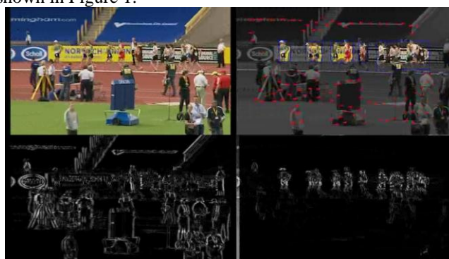
Figure 1: Matching of key-points in successive frames (top-right crosses), cluttered frame difference (bottom-left) and projectively matched frame difference (bottom-right) showing potential athletes. Detected bodies are marked by blue rectangles (top-right)
